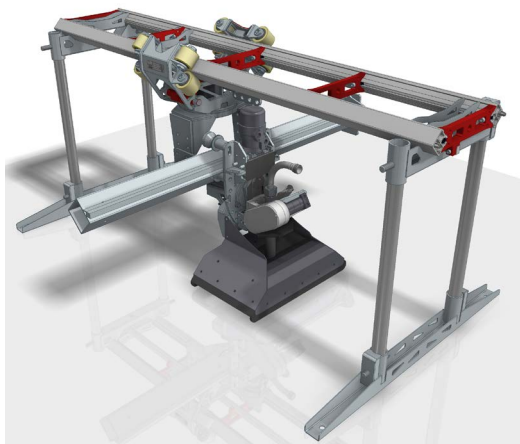
The spine roller is connected to the spine rail with a single bolt.
