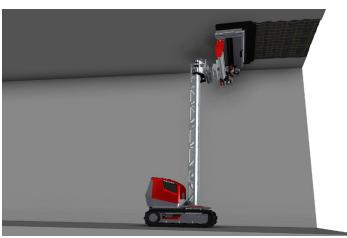
The Aqua Cutter 450V, equipped with an extendable tower system, is the perfect choice for vertical applications in tight spaces such as shafts, high walls, and overhead work, but it is just as efficient in horizontal work. It offers a reach of up to 4 meters (13.1 feet) without support and up to 10 meters (32.8 feet) with support. Its adjustable hoist and tilt function ensure precise positioning of the power head, making it easy to retract, inspect the results, and resume work seamlessly.
