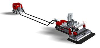
With a disconnectable Power Control Module (PCM), both Aqua Cutter 450 models can reach areas inaccessible to electric-powered equipment. Separating the PCM from the tracked crawler allows them to operate independently via radio control. This keeps the PCM in a safe location while the fully submersible crawler navigates confined or hazardous spaces, such as narrow tunnels or flooded sewer pipes.
