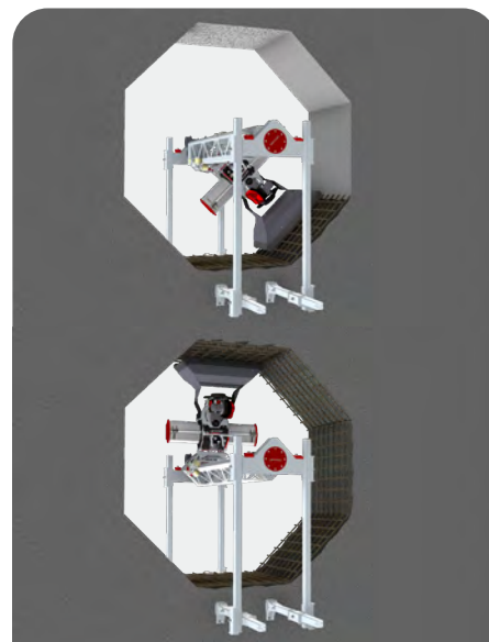
With a rotational Spine, it's easy to adjust the Power head to different surface angles.
