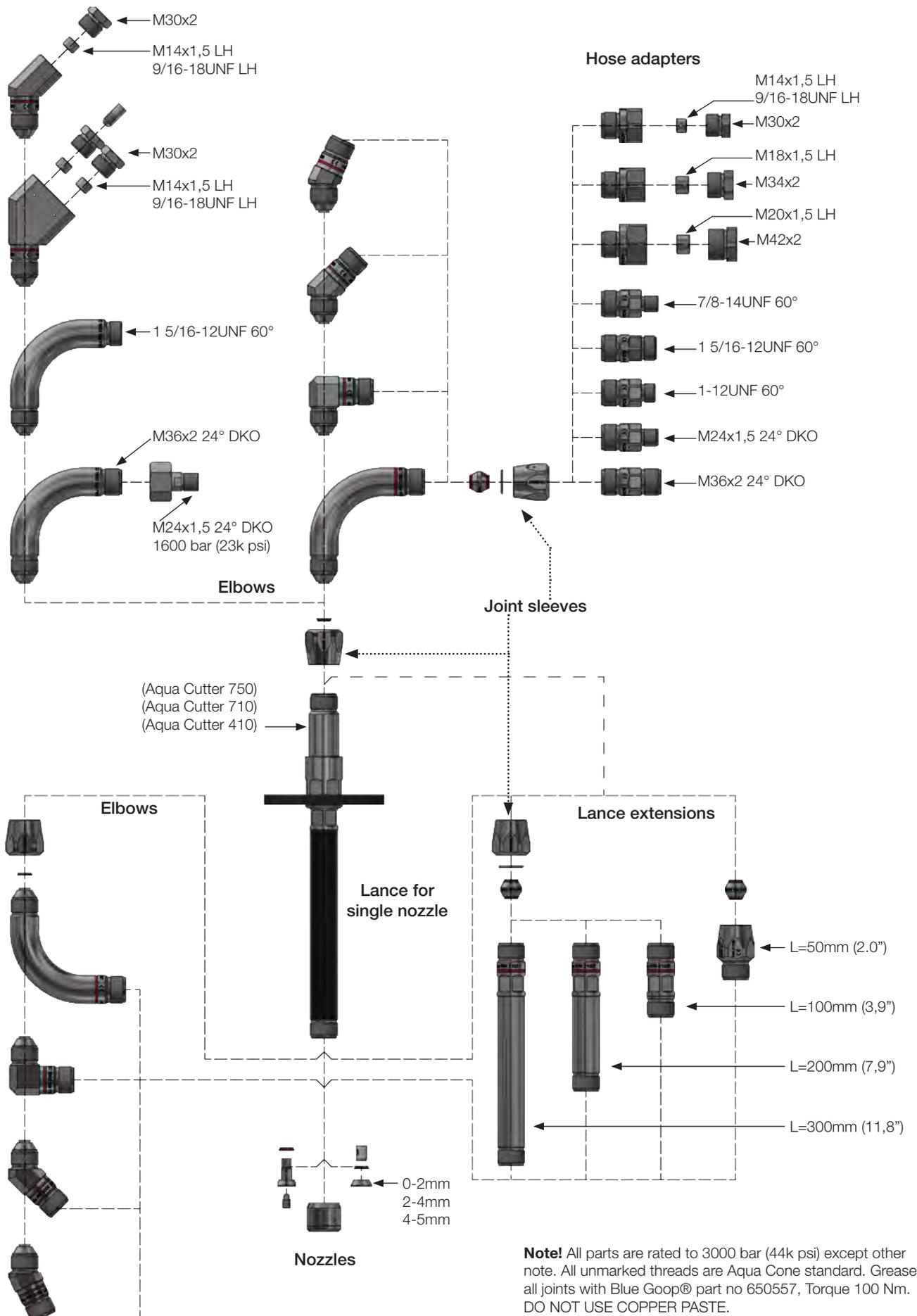
**Note!** All parts are rated to 3000 bar (44k psi) except other note. All unmarked threads are Aqua Cone standard. Grease all joints with Blue Goop® part no 650557, Torque 100 Nm. DO NOT USE COPPER PASTE.
